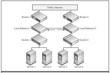
Figure 1-2. Load balancing example (courtesy of Rackspace.com)
